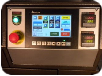
Delta PLC with 40 program memory and self-diagnostics
